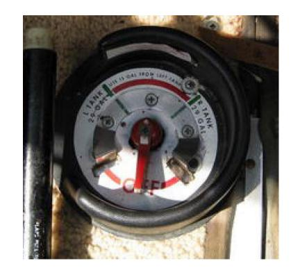
The failure to comply with an airworthiness directive (AD) by maintenance personnel and incorrect reinstallation of the fuel selector handle by unknown personnel, which resulted in fuel starvation
