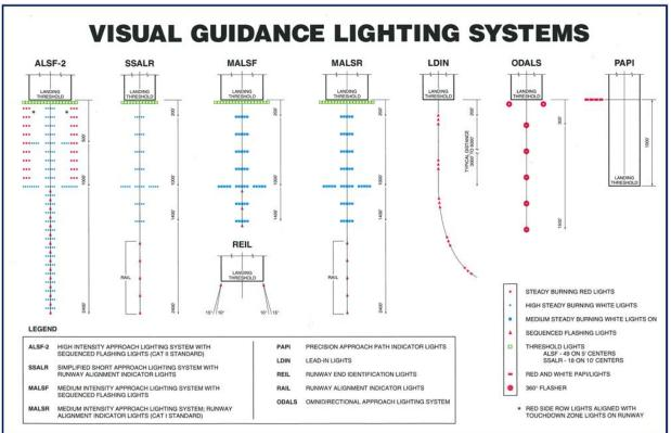
Figure 22: Existing Configurations of Approach Lighting Systems (ALS)
