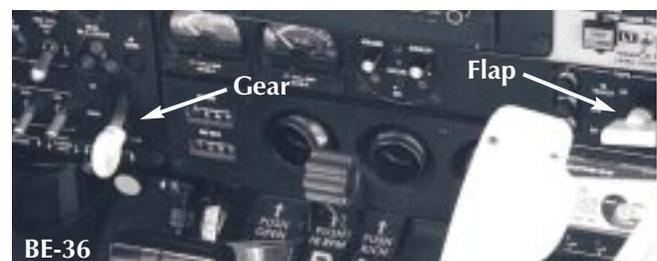
During landing rollout, while turning off the runway, the pilot inadvertently selected gear up on the BE-35 aircraft. The pilot, who owns a similar aircraft, had borrowed this aircraft. The gear and flap controls on the pilot's aircraft are in the opposite position of those in the borrowed aircraft. The pilot intended to raise the flaps, not the gear.
