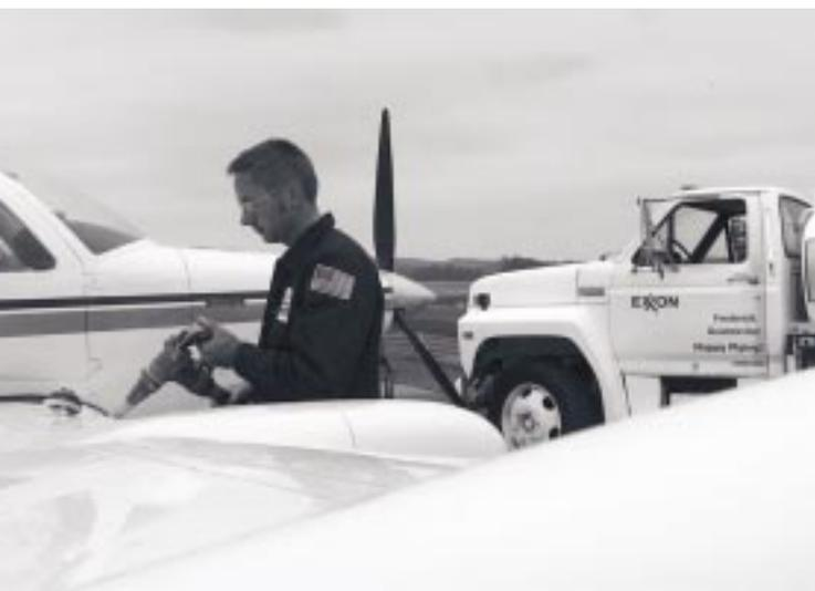
Review the fuel system for the aircraft you fly. Prior to 1961, many BE-35s had two main wing tanks and one or two auxiliary tanks. There was a single fuel gauge with a left/right selector switch to monitor fuel on board. Later models differ from earlier models. Consult the POH for the aircraft you fly.
