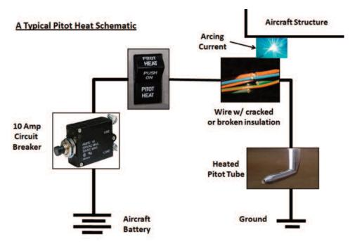
The purpose of a circuit breaker is to open the circuit if the current draw exceeds the rated amperage (due, for example, to an exposed wire coming into contact with another damaged wire, or the aircraft structure). This stops the flow of electricity, preventing further damage or fire hazard.
